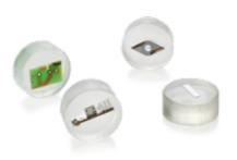
The Qmount is a modern device for the lightcuring-based mounting of materialographic samples.
